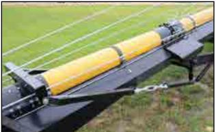
Fig 88 - Under-bridging turnbuckle on some units
