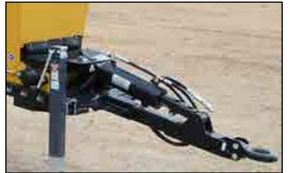
Fig 53 - Hydraulic hitch
