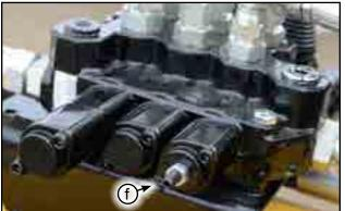
Fig 47 - Valve adjustment, rear of bank
