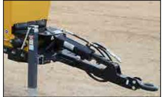
Fig 35 - Hydraulic hitch
