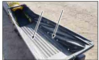
Fig 74 - Open transition hopper flashing
