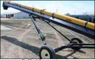
Fig 30 - A-Frame undercarriage
