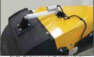
Fig 27 - Discharge spout with electric actuator
