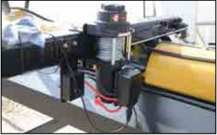
Fig 51 - Electric winch
