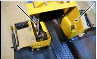
Fig 58 - Hold-down wheel location
