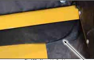
Fig 108 - New side flashing
