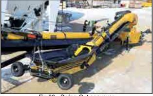
Fig 36 - Swing-Out conveyor
