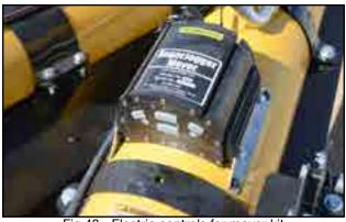
Fig 48 - Electric controls for mover kit
