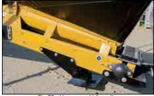
Fig 77 - Hopper and idler roller
