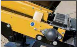
Fig 89 - Idler roller adjustment bolt
