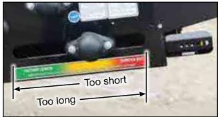
Fig 59 - "Slack Eliminator" roller. Belt length indication
