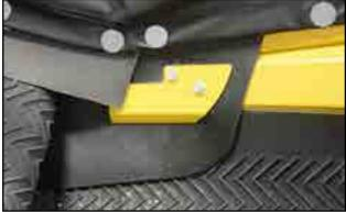
Fig 115 - Fasten flashing clamp
