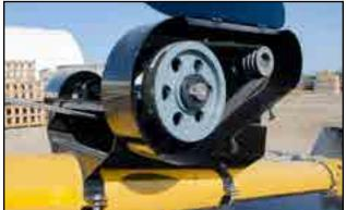
Fig 119 - Motor-to-Countershaft belt
