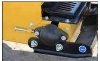
Fig 94 - Hopper idler roller bearing
