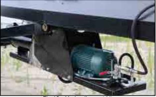
Fig 12 - Hydraulics wet kit
