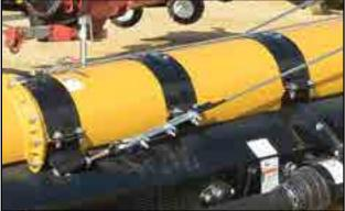
Fig 86 - Eyebolts and cable bridging
