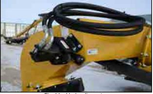
Fig 44 - Hydraulic motor
