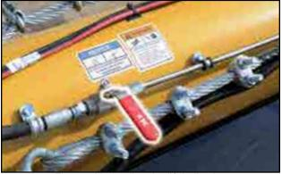
Fig 52 - Hydraulic tube lift ball valve
