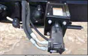
Fig 13 - Hydraulic motor
