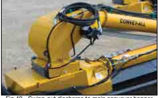
Fig 40 - Swing-out discharge to main conveyor hopper
