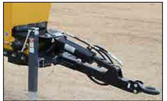
Fig 60 - Hydraulic hitch
