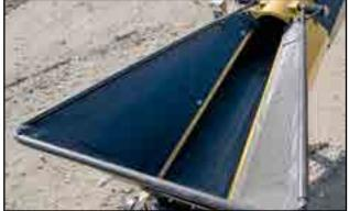
Fig 109 - Completed hopper with belt
