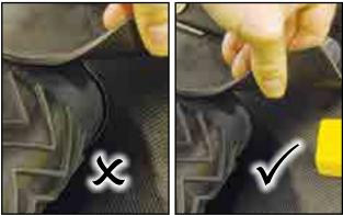
Fig 114 - Corner flashing must fit tight around the belt
