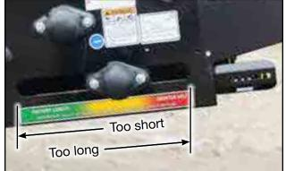
Fig 90 - "Slack Eliminator" roller. Belt length indication
