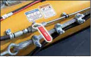
Fig 18 - Hydraulic valve to conveyor tube cylinders
