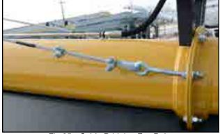
Fig 85 - Cable Bridging Eye Bolts
