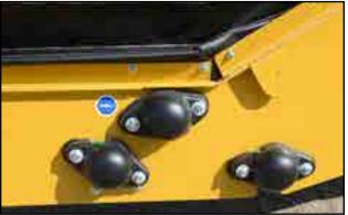
Fig 78 - Transition roller bearings
