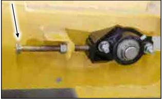
Fig 93 - Open transition hopper adjustment bolt
