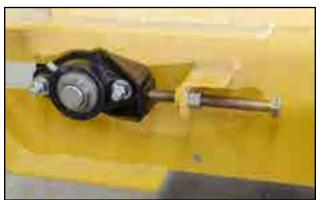
Fig 99 - Idler roller bearing on the swing-out
