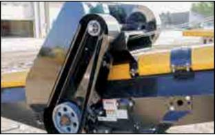
Fig 117 - Drive-to-Countershaft belt
