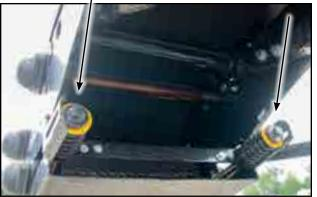
Fig 71 - Tension bolts, Spring Tension Drive Box
