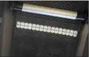
Fig 69 - Belt lacing and roller
